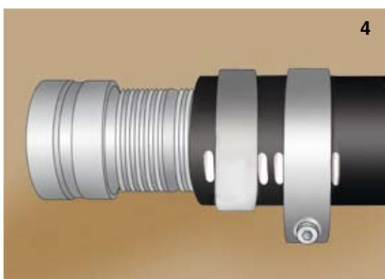
4. Insert fitting all the way into the hose. A soft hammer can be used to tap hose tails into place.
