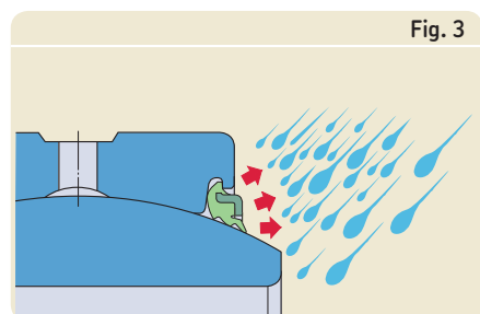
Three seal lips keep contaminants out
