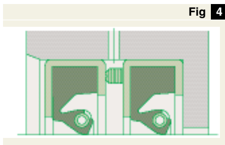
Radial shaft seals of the HDS design mounted adjacent to each other
