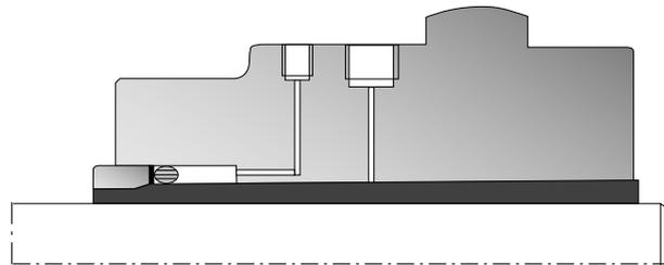
Integrated OK coupling system in existing gear hubs.
