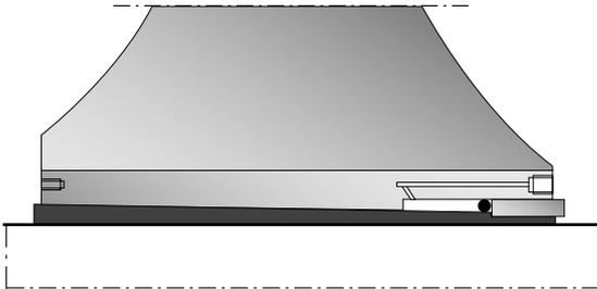
Double sleeves system OKD for keyless connections of large hubs.
