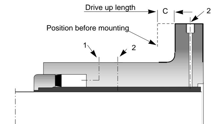
1. One BSP 1/4 connection hole for pump and one BSP 1/4 vent hole for air release
