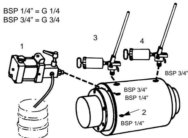
For OKC 180 – OKC 190: After the initial mounting operation, release the horizontal grub screws, and then tighten the coupling nut firmly. Retighten the grub screws.
