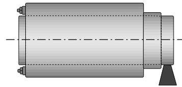
Note: during this process the coupling must not weigh upon the shaft.
