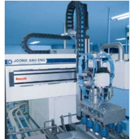
The camoLINE modular system: the quick and easy method to create an application-specific handling system
