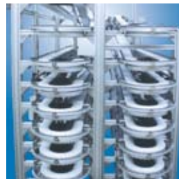
Alpine conveyor buffer system
